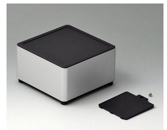
ES126059 SYNERGY S120 Aluminium AlMgSi 0.5 matt anodised 120x120x70mm IP 40
