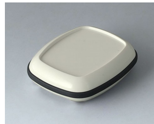
B1604217 BODY-CASE M, with recess ASA (UL 94 HB) traffic white RAL 9016 50x41x14mm IP 65
