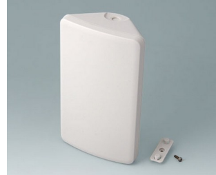
B4610107 SMART-CONTROL M, Vers. I ASA+PC (UL 94 V-0) off-white RAL 9002 173x101x59mm IP 40, IP 55 opt.
