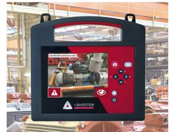
Diagnostic camera for illustrating the machine status
