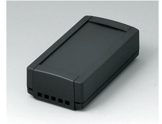
B1040469 TOPTEC 102, Vers. II ABS (UL 94 HB) black RAL 9005 102x54x30mm IP 40
