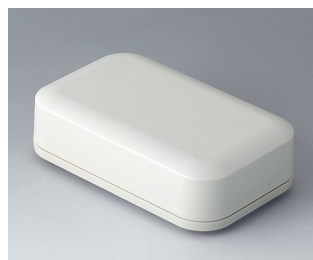
A9433107 EVOTEC 125, Vers. I ASA+PC-FR (UL 94 V-0) off-white RAL 9002 125x78x37mm IP 65 opt., IP 40
