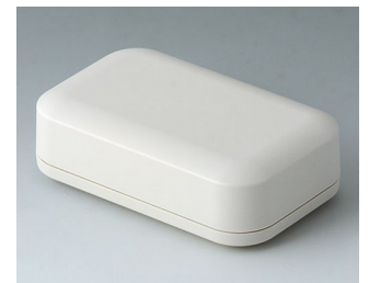
A9423107 EVOTEC 100, Vers. I ASA+PC-FR (UL 94 V-0) off-white RAL 9002 100x62x31mm IP 65 opt., IP 40
