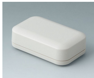
A9403107 EVOTEC 80, Vers. I ASA+PC-FR (UL 94 V-0) off-white RAL 9002 80x50x26mm IP 65 opt., IP 40
