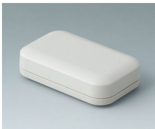
A9401107 EVOTEC 80, Vers. I ASA+PC-FR (UL 94 V-0) off-white RAL 9002 80x50x22mm IP 65 opt., IP 40
