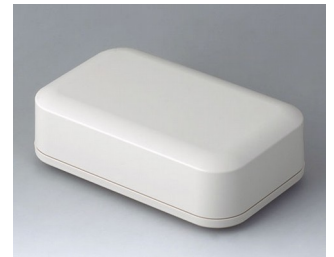
A9443107 EVOTEC 150, Vers. I ASA+PC (UL 94 V-0) off-white RAL 9002 150x93x45mm IP 65 opt., IP 40
