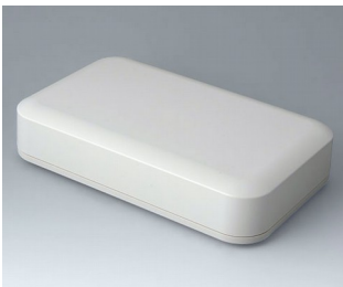
A9481107 EVOTEC 250, Vers. I ASA+PC-FR (UL 94 V-0) off-white RAL 9002 250x155x54mm IP 65 opt., IP 40
