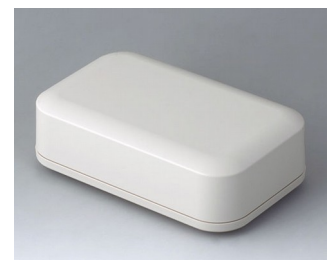
A9443107 EVOTEC 150, Vers. I ASA+PC-FR (UL 94 V-0) off-white RAL 9002 150x93x45mm IP 65 opt., IP 40
