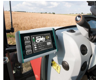
ISOBUS terminal for tractors and self-propelled machines
