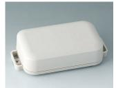
C3207207 EASYTEC 125 ASA+PC (UL 94 V-0) off-white RAL 9002 147x78x37mm IP 65 opt., IP 40
