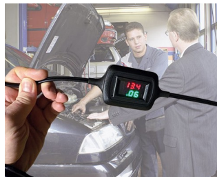
Voltage and current display during trickle charging
