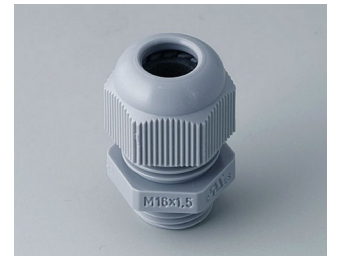
C2316418 Cable gland M16x1.5 PA 6 silver grey RAL 7001 IP 68
