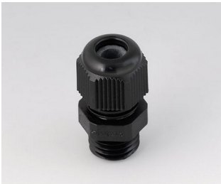
C2312419 Cable gland M12x1.5 PA 6 black RAL 9005 IP 68
