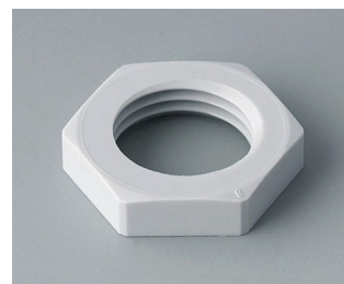
C2316117 Counter nut M16x1.5 PA 6 light grey RAL 7035
