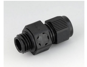
C2312919 Cable gland M12x1.5, pressure compensation PA 6 (UL 94 V-0) black RAL 9005 IP 68
