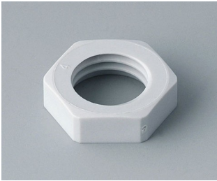
C2312117 Counternut M12x1.5 PA 6 light grey RAL 7035
