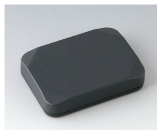
B1824118 MINI-DATA-BOX E50, flat ASA+PC (UL 94 V-0) anthracite grey RAL 7016 70x50x15mm IP 65 opt., IP 40
