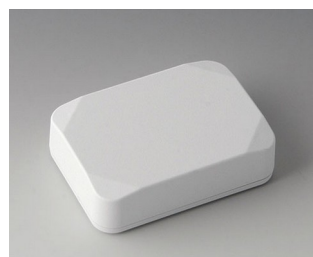
B1824217 MINI-DATA-BOX E50, high ASA+PC (UL 94 V-0) traffic white RAL 9016 70x50x20mm IP 65 opt., IP 40
