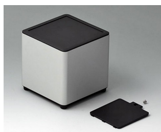
ES109059 SYNERGY S100 Aluminium AlMgSi 0.5 matt anodised 100x100x100mm IP 40
