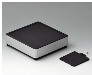
ES143059 SYNERGY S140 Aluminium AlMgSi 0.5 matt anodised 140x140x40mm IP 40
