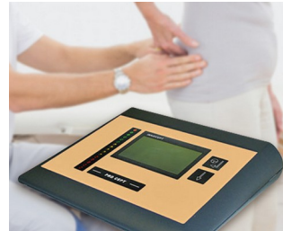
EMG bio-feedback for incontinence diagnostics and therapy
