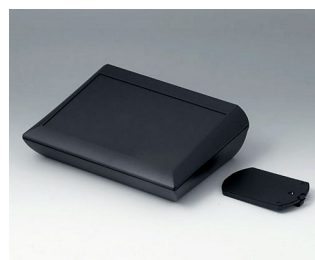
A0620119 COMTEC 200 H, Vers. II ABS (UL 94 HB) black RAL 9005 200x150x62.8mm IP 40
