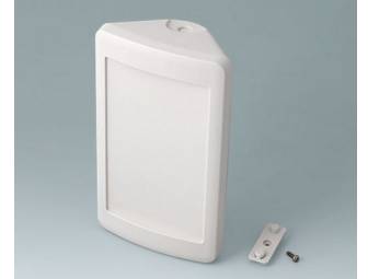
B4610207 SMART-CONTROL M, Vers. II ASA+PC (UL 94 V-0) off-white RAL 9002 173x101x59mm IP 40, IP 55 opt.
