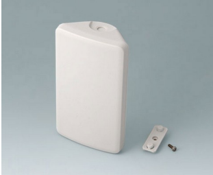
B4608107 SMART-CONTROL S, Vers. I ASA+PC (UL 94 V-0) off-white RAL 9002 142x81x46mm IP 40, IP 55 opt.
