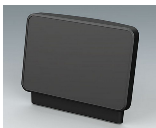
C3604408 Operating panel M ASA+PC (UL 94 V-0) anthracite grey RAL 7016 328x78x275mm
