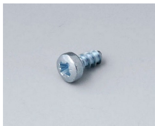
A0306031 Self-tapping screws 3 x 6 mm (PZ1)
