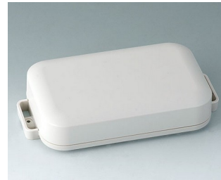
C3208107 EASYTEC 150 ASA+PC (UL 94 V-0) off-white RAL 9002 172x93x36mm IP 65 opt., IP 40
