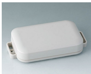
C3207107 EASYTEC 125 ASA+PC (UL 94 V-0) off-white RAL 9002 147x78x30mm IP 65 opt., IP 40
