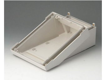
B4016217 DATEC-TERMINAL M, Vers. II ABS (UL 94 HB) off-white RAL 9002 168x272x101mm IP 54 opt.
