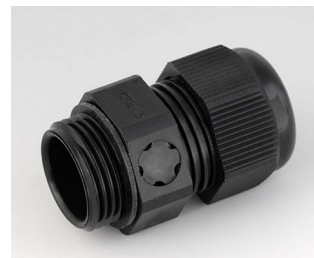
C2320919 Cable gland M20x1.5, pressure compensation PA 6 (UL 94 V-0) black RAL 9005
