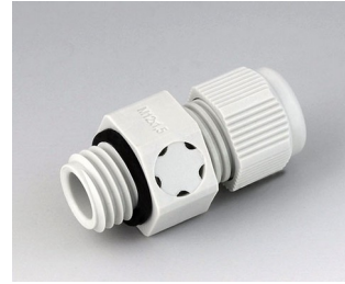
C2312917 Cable gland M12x1.5, pressure compensation PA 6 (UL 94 V-0) light grey RAL 7035 IP 68
