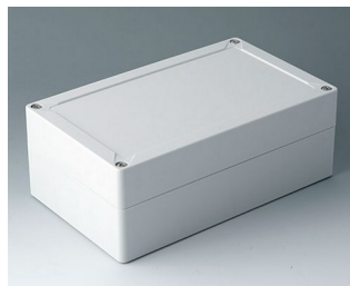
C7020042 IN-BOX PC light grey RAL 7035 202x122x75mm IP 66, IP 67, IK 08
