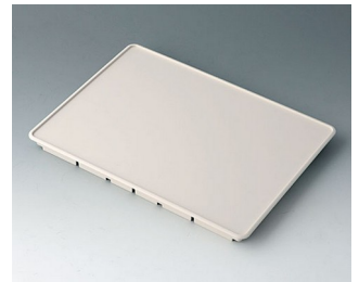
B4144107 Front panel M ABS (UL 94 HB) off-white RAL 9002 225.6x165.6x15.5mm
